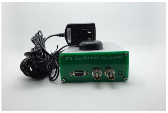
Keep GPSDO running about 24Hours, it will getting very stable 10MHz. it need a little bit long time to download GPS data(30min-2Hours).
